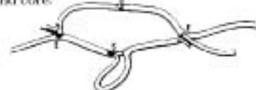
5. Insert taped end of one core into the fid socket. Insert fid at point "S" on the other rope jacket. With the pusher, push fid through the center of the jacket and bring it out at point "E". Repeat this procedure with the other core and jacket.
