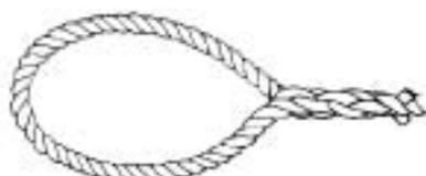
4. Pull each strand snugly up to the main body of the rope then tuck them, in sequence, over and under the strands in the rope. While it is traditional to use 4 tucks, at least 6 tucks are recommended for synthetic fiber ropes.
