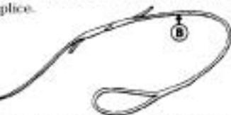
4. Splice end B into original rope with an End-to-End splice.
