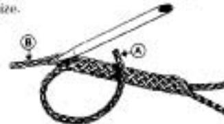
3. Splice A into B as described in End-To-End splice.
