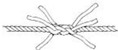
3. Remove the temporary tie and make two tucks with the other three strands. You now have the strands of each rope tucked two times through the strands of the other rope. Now go back and make at least two more tucks with each of the six strands . . . four additional tucks are recommended for synthetic ropes.
