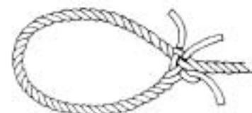
3. Tuck the last unlaidd strand under the remaining strand in the rope, making sure the tuck is against the twist.
