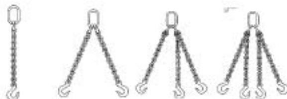
Single Leg Sling    Double Leg Sling    Triple Leg Sling    Quadruple Leg Slings
