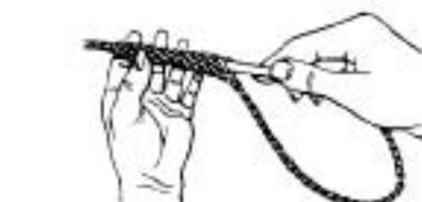
3. As fid penetrates strands, guide the fid down the hollow center of the rope. In this step, push fid with right hand . . . at the same time use left hand to work the rope over the fid.
