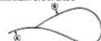
1. Cut approximately 2 ft. from one end of rope to be spliced. Put end B into splicing fid and insert it about 8 inches from one end of rope. Push fid 4 inches through center of rope and bring it out., leaving end approximately 4 inches long.
