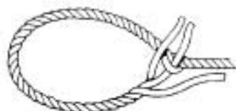
1. To begin your Eye Splice unlay the strands for a short distance and double back to form a loop of the desired size, with the unlaidd strands laying across the twist of the rope.
