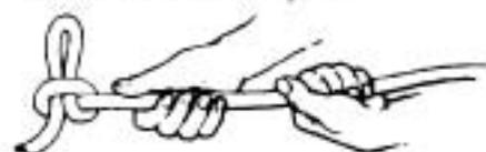
6. Remove tape from jacket ends and pull crossover snug by pulling jacket and core simultaneously on each side of splice. Hold the crossover firmly and smooth excess braid away from it in both directions. Cut off protruding cores at point "E".
