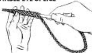
1. Insert rope into hollow end of splicing fid, then insert fid into rope at point about 24 inches from its end. As fid penetrates strands, guide it down the hollow center of the rope. In this step, push fid forward with right hand . . . at the same time use left hand to work the rope over the fid.
