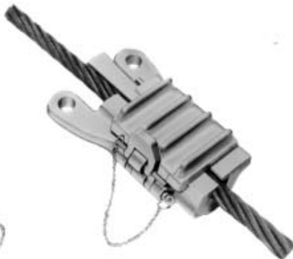
Cable can be released while under full tension by releasing latch on hinged lid. Lid is securely latched and locked with pin while in use.
