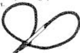
2. Start splice two stitches above penetrating rope. Run fid through penetrating rope and continue down the hollow center for approximately six inches. Bring fid out through stitches. Remove from rope.
