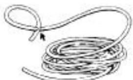
2. Remove fid and pull entire length of rope through to size of Eye splice desired.
