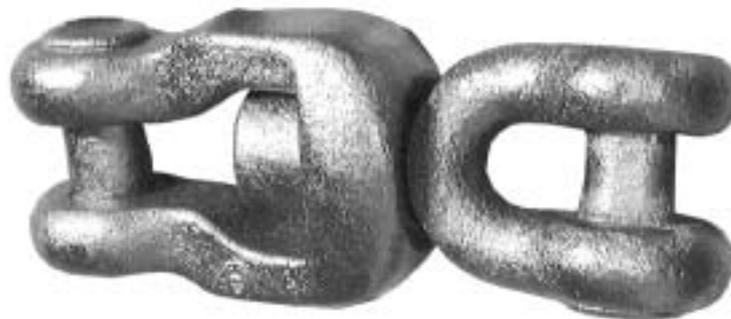
The Jaw & Jaw swivel shackle is designed to accept the shank of an anchor and the chain end is designed to accept a closed spelter socket or mooring chain.
