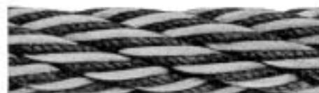
Spring-Lay is used for marine towing and mooring lines. High in strength—for strength equal to manila rope it only needs to be one-half the diameter, and its weight is less than manila rope of equal strength.
