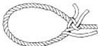
2. The next unlaidd strand going over the strand under which the center unlaidd strand is tucked, and is tucked under the next strand in the rope.
