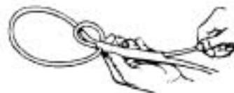
3. Tighten splice. Clip protruding end.
