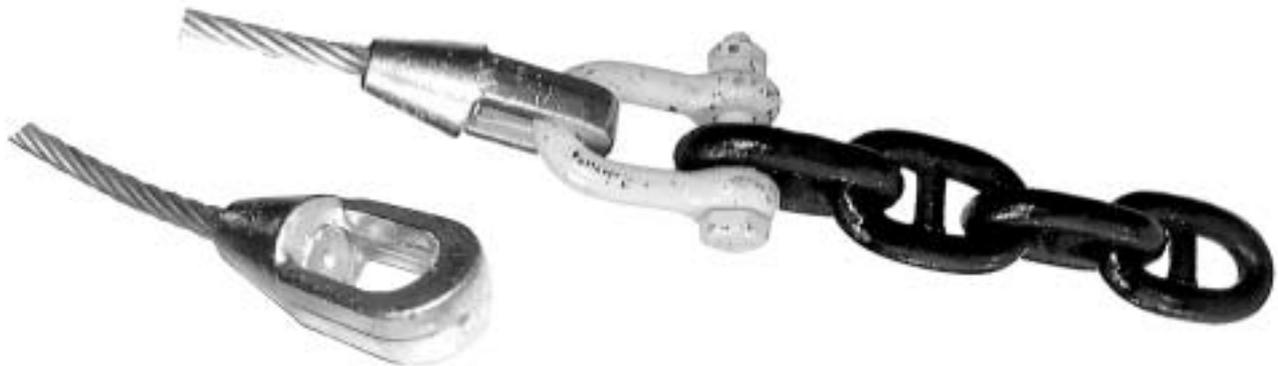
MARQUIP round-to-round special towing sockets are designed to eliminate excessive wear at contact points. They provide superior safety and longer service under heavy tows using 2" to 2-1/8" cable. They can also be modified to accept 2-1/4" extra-improved plow steel wire rope, with no reduction in reliability.
